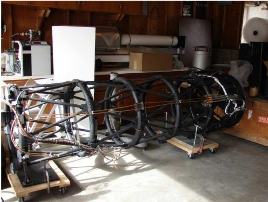
This is the society's newest telescope, a 26-inch reflector that was originally designed and built to go on a spacecraft, then used at the Big Bear Solar Observatory for solar work. We think the truss is steel, aluminum and titanium, and was designed to focus view motors (hence the wiring). To get some idea of the size of this thing, see the image below.
