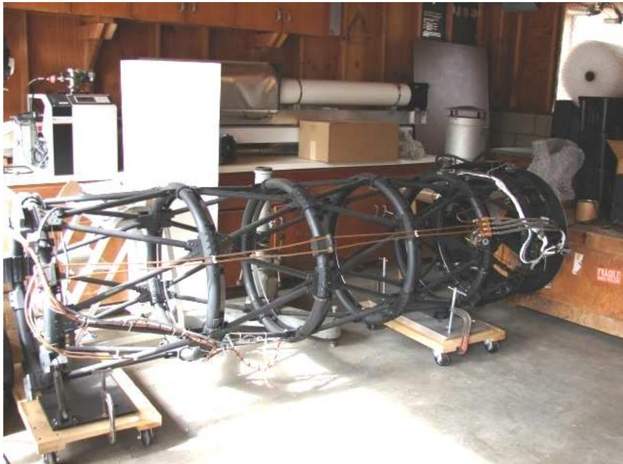
This is the reflector at Big Bear prior to The Move. You can't get a real sense of its size. All that tubing is steel, not aluminum. Despite this, the telescope is much lighter than one would expect. Note all that wiring; the scope even had remote controlled focusing ! This image and all others courtesy of Minghua Nie.
