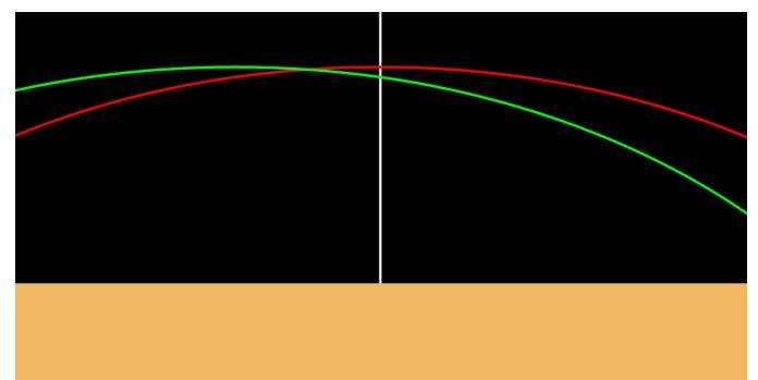
The illustration above shows the opposite situation, with the mount pointed a little to the west of true north. Now the mount will track gradually south of where it should, and the star drifts north. Then the adjustment is to move the mount's azimuth a little to the east.
