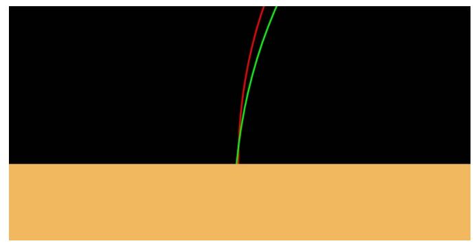
If the mount is pointed higher than true north, then the green line is where the mount's celestial equator is. In this case, the mount gradually tracks further south than it should, and the star drifts north, so you have to adjust your polar axis to point lower.
