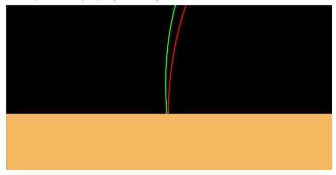
The reverse happens if the mount were pointed too low. Then your mount's celestial equator is tilted higher than it should be, as shown above. Now the star drifts to the south, so you adjust the polar axis a little higher than it is.
