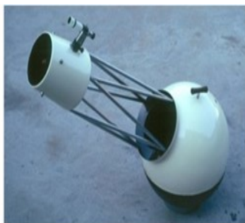
8" f/7 Newtonian in 24" Ø Sphere - Also shown in TM1
