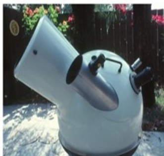
8" f/4.5 Newtonian final Remount in 20" Ø Sphere - Featured in TM2
