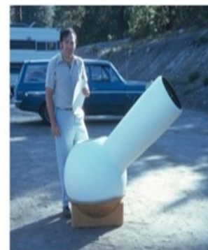
12-1/2" f/5 RFT First Light – Mt.Pinos and Sunland, CA Make parts TM3 Ass'y TM4
